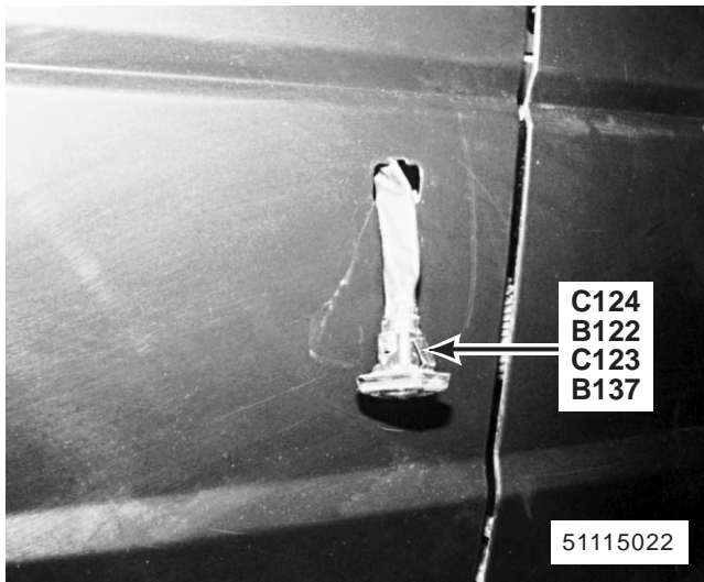
25. LH front side of vehicle (RH similar) B122 Left Repeater Lamp B137 Right Repeater Lamp C123 (2-B) (Right) C124 (2-B) (Left)
