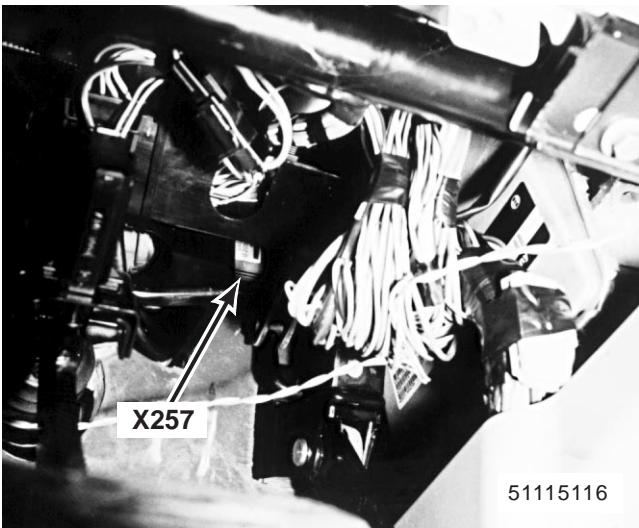
123. behind RH side of fascia right of steering column X257 Throttle Position Sensor
