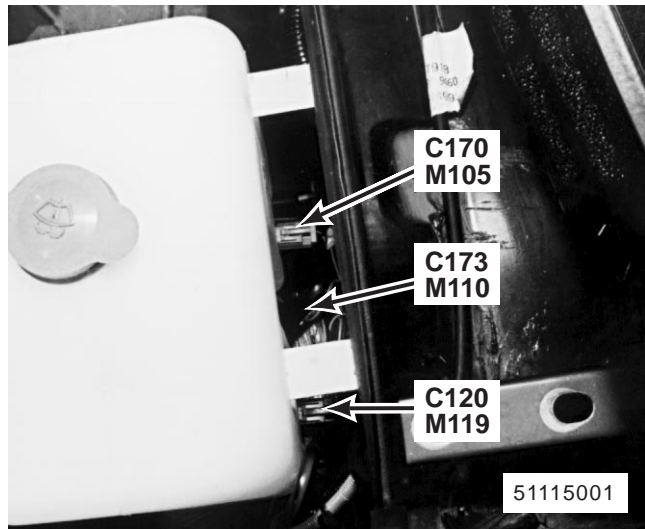
2. LH rear of engine compartment M105 Front Screen Wash Pump M110 Headlamp Wash Pump M119 Rear Screen Wash Pump C120 (2-B) C170 (2-R) C173 (2-B)
